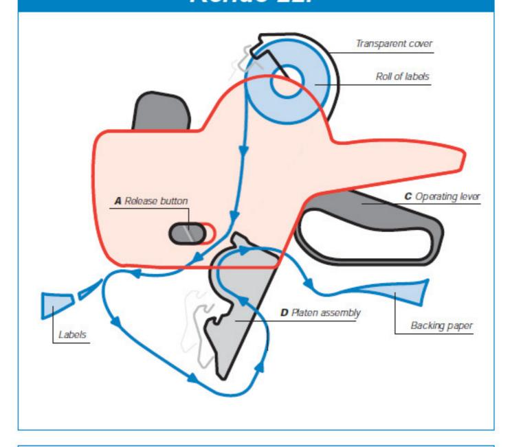
Lift transparent cover and place roll of labels into the machine.
